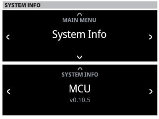
"System Info" displays information about current MCU, LCD and FPGA firmware versions.
