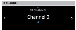
The C 399 has the capability to operate via Alternate IR channel. This is useful if you have two NAD products that can be operated by similar remote control commands. With alternate IR Channel, two different NAD products can be controlled independently in the same zone by setting each one to a different IR channel.
